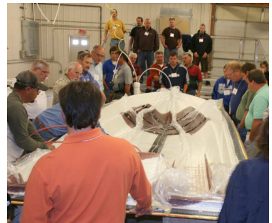
Participants observe as red fiberglass resin is pulled across the mold of a boat hull during the vacuum infusion process at Carstens Industries.
