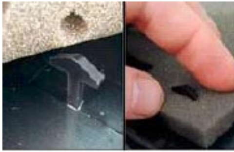
A dart connector, which replaces the use of an adhesive, holds acoustic foam securely in place on the inside of an IBM computer front panel.
