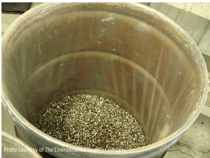
Figure 6: Mercury containing pellets in drum.
